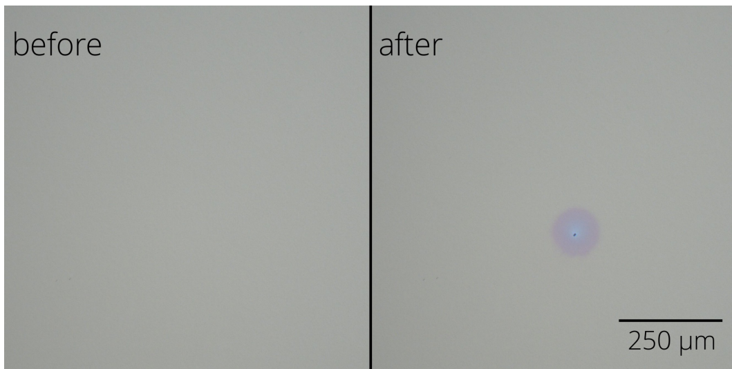
Figure 4. Typical damage morphology: fluence 60.7 J/cm 2 , damage after 100 pulse(s) in fluence level.
