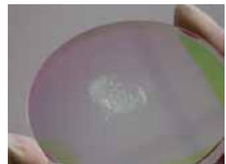
Surface Damage Failure Mode: Contaminations
