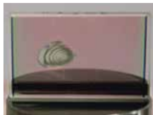
Surface Damage Failure Mode: Light Absorptance & Fatigue
