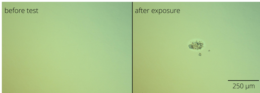
Figure 4. Typical damage morphology: irradiance 1.41 MW/cm 2 , exposition time 1 ms.
