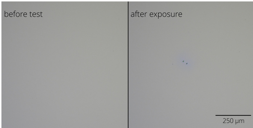
Figure 5. Typical damage morphology: fluence 21.9 \text{ J/cm}^2 , damage after 1 pulse(s).
