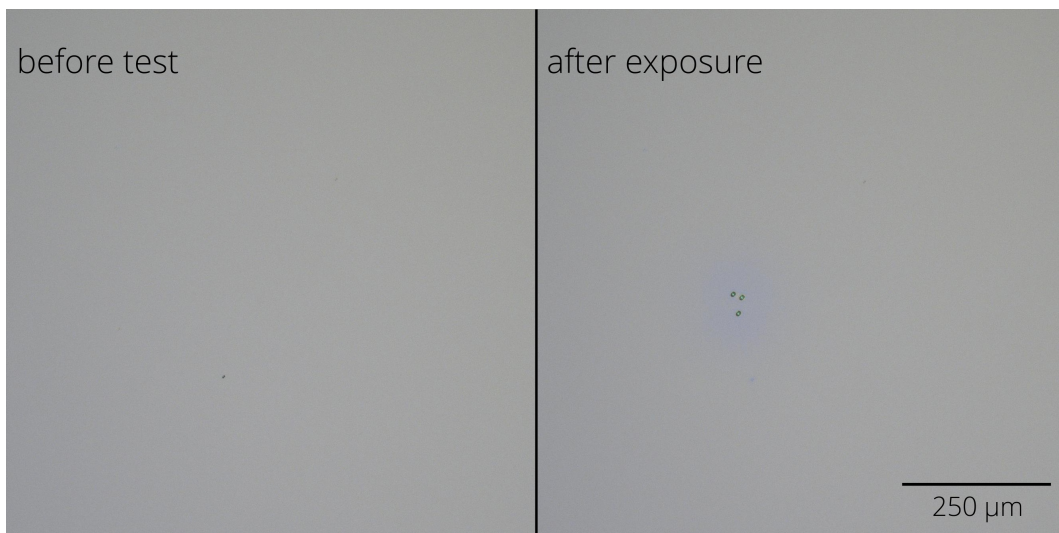
Figure 6. Typical damage morphology: fluence 26.1 \text{ J/cm}^2 , damage after 1 pulse(s).
