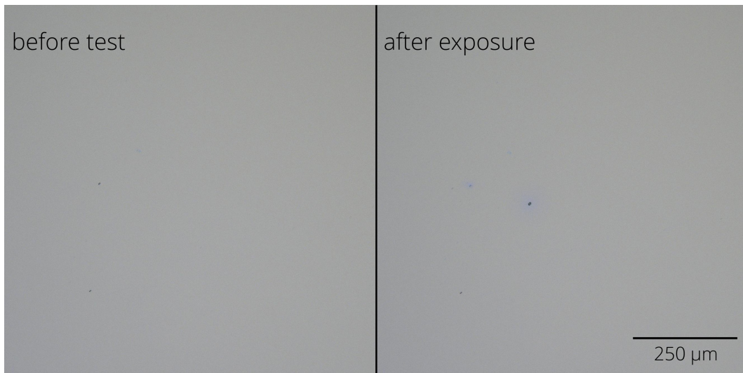
Figure 4. Typical damage morphology: fluence 17.9 \text{ J/cm}^2 , damage after 1 pulse(s).
