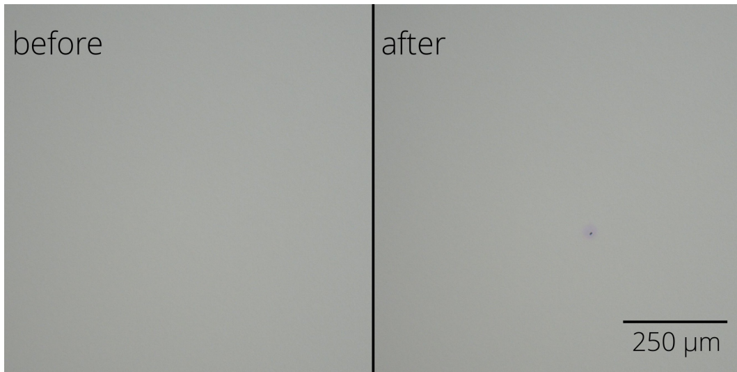
Figure 5. Typical damage morphology: fluence 60.8 \text{ J/cm}^2 , damage after 100 pulse(s) in fluence level.
