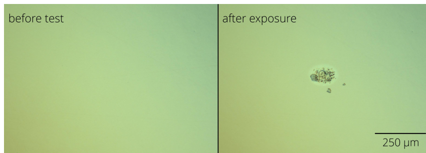
Figure 4. Typical damage morphology: irradiance 1.41 \text{ MW}/\text{cm}^2 , exposition time 1 ms.
