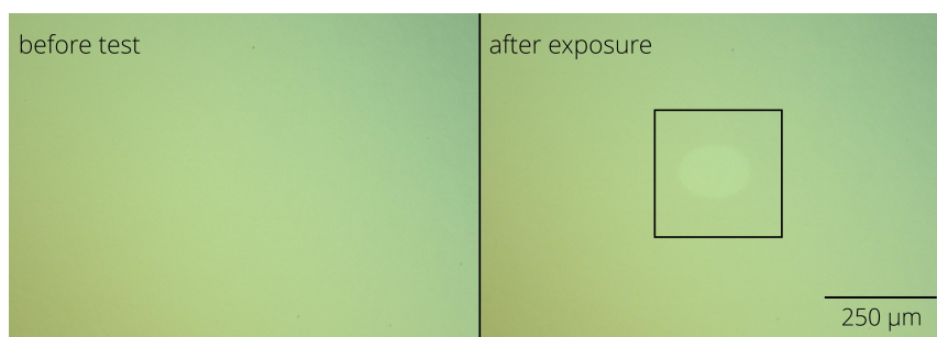
Figure 8. Typical damage morphology: irradiance 0.813 MW/cm 2 , exposition time 30.0 s.
