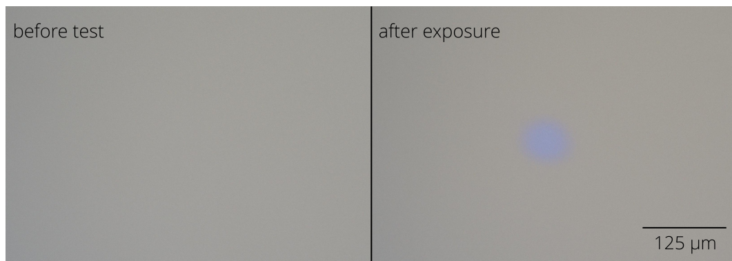
Figure 9. Typical damage morphology: fluence 0.402 \text{ J/cm}^2 , damage after 1000000 pulse(s).
