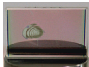
Surface Damage Failure Mode: Light Absorbance & Fatigue
