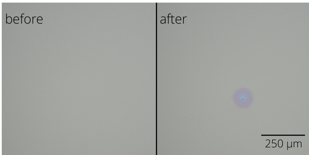
Figure 4. Typical damage morphology: fluence 60.7 \text{ J/cm}^2 , damage after 100 pulse(s) in fluence level.
